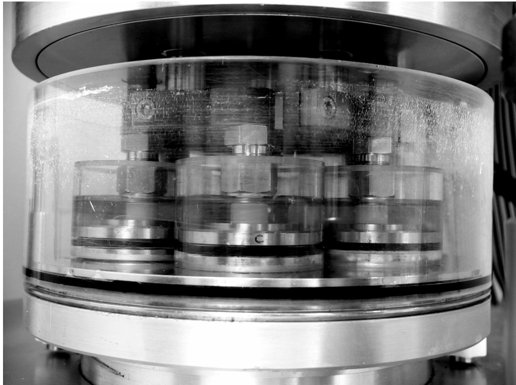
Figure 3: Experimental set-up showing OrthoPOD™ (Advanced Mechanical Technology, Inc., Watertown, MA) 6-station multi-directional wear tester.
