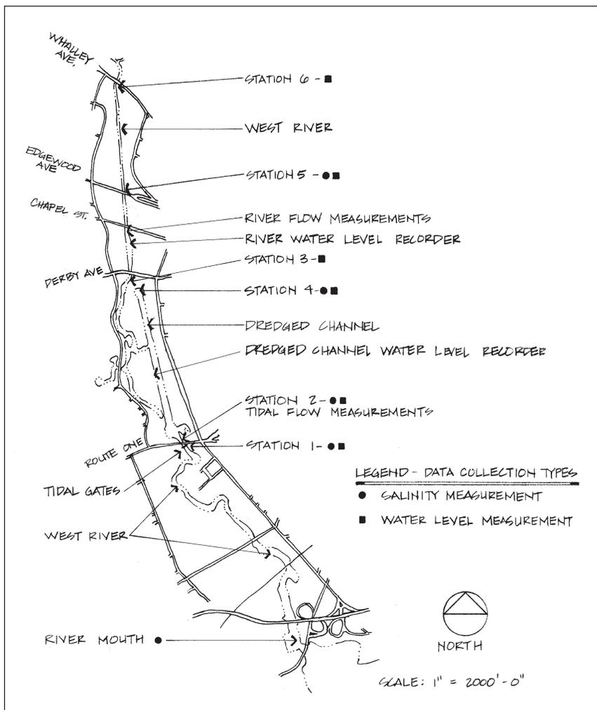
Figure 2. Sampling stations for water level, salinity, and flow in the West River Marsh, New Haven, Connecticut. Solid circles indicate sites of salinity measurements. Solid squares indicate the location of staff gauges for water level measurements.
