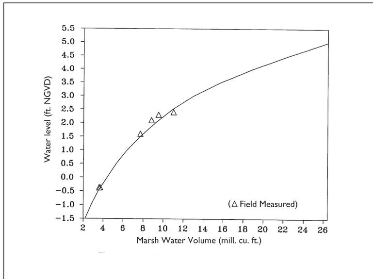
*Close agreement between the equation derived from topographic data and volume calculations and data points developed independently from field measurements validates the accuracy of the regression model.*
