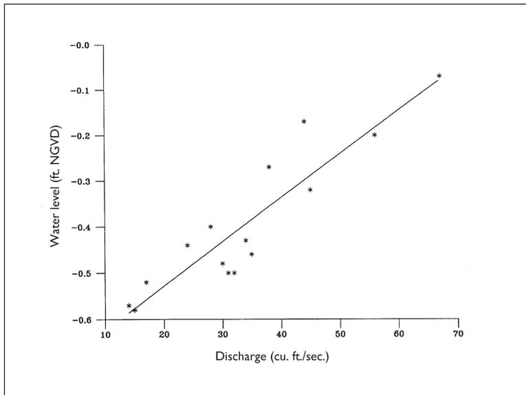
Figure 6. Rating curve for baseflow conditions on the West River south of the Chapel Street bridge, New Haven, Connecticut.
