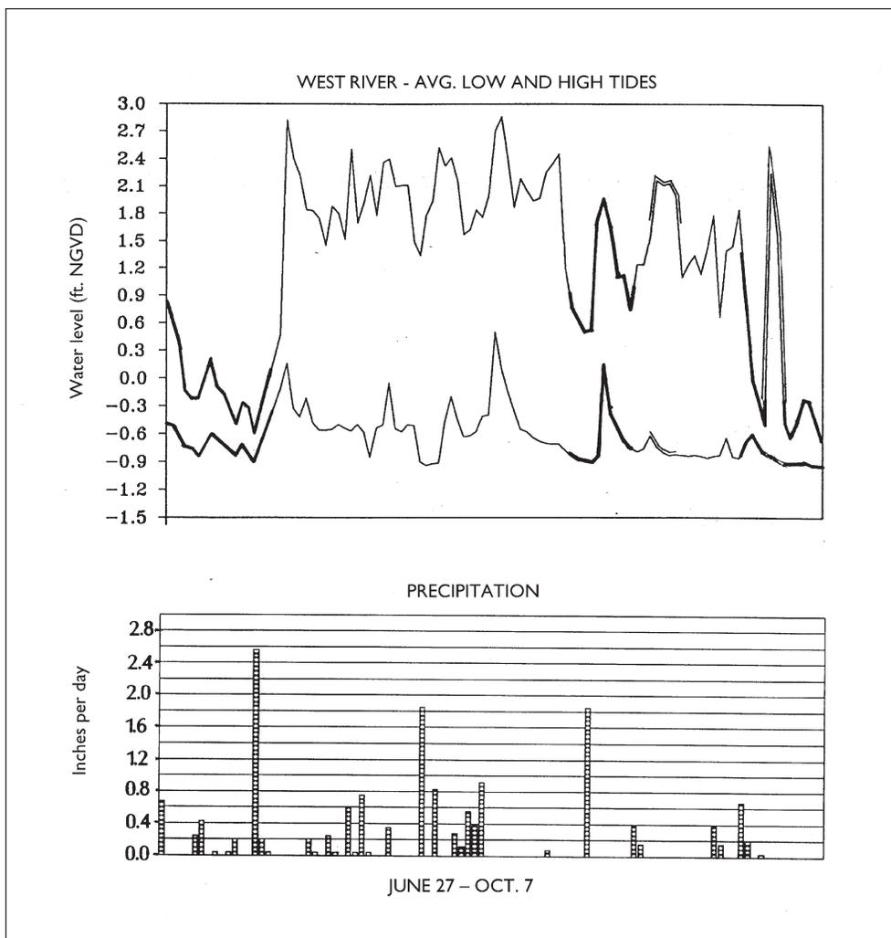
Figure 3. (a) Mean low and high water level in the West River marsh between Chapel Street and Derby Avenue for the period June 27 to October 7, 1992 with all tide gates closed (dark solid line), one gate open (solid line), and two gates open (double line); (b) histogram of daily rainfall.
