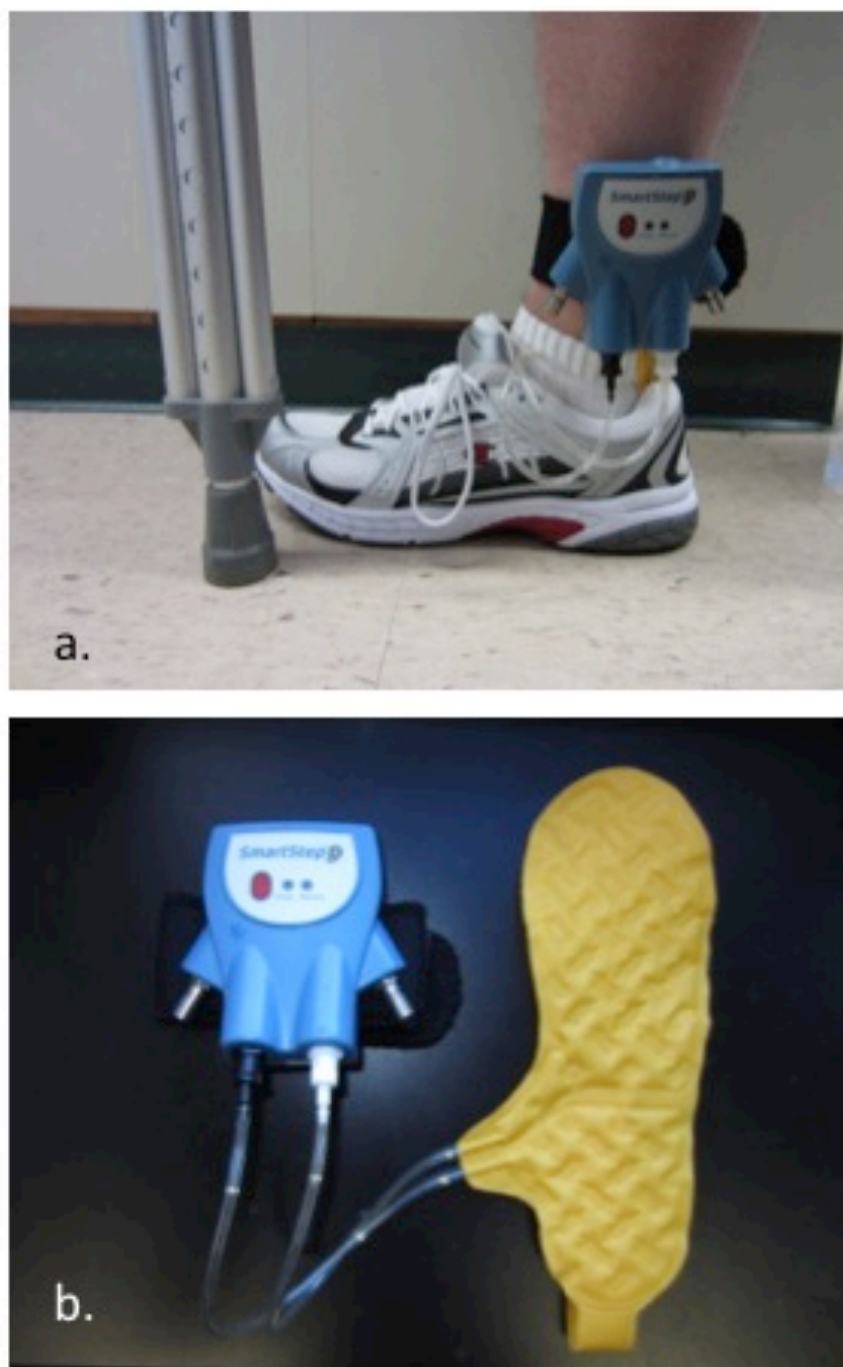
Figure 5. a. Placement of the SmartStep device with insole in standard shoe and transmitter strapped around the ankle. b. SmartStep equipment including transmitter and insole.
